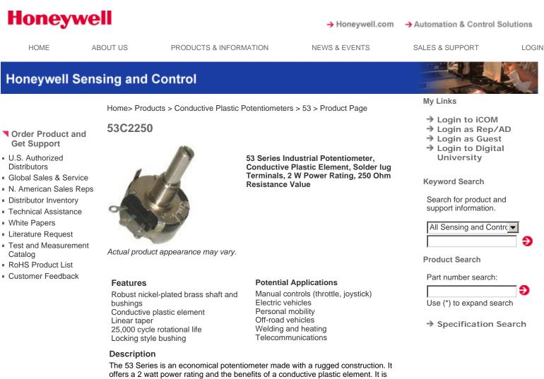
offers a 2 watt power rating and the benefits of a conductive plastic elemen available in a special construction that accepts a rotary switch (purchased separately).
